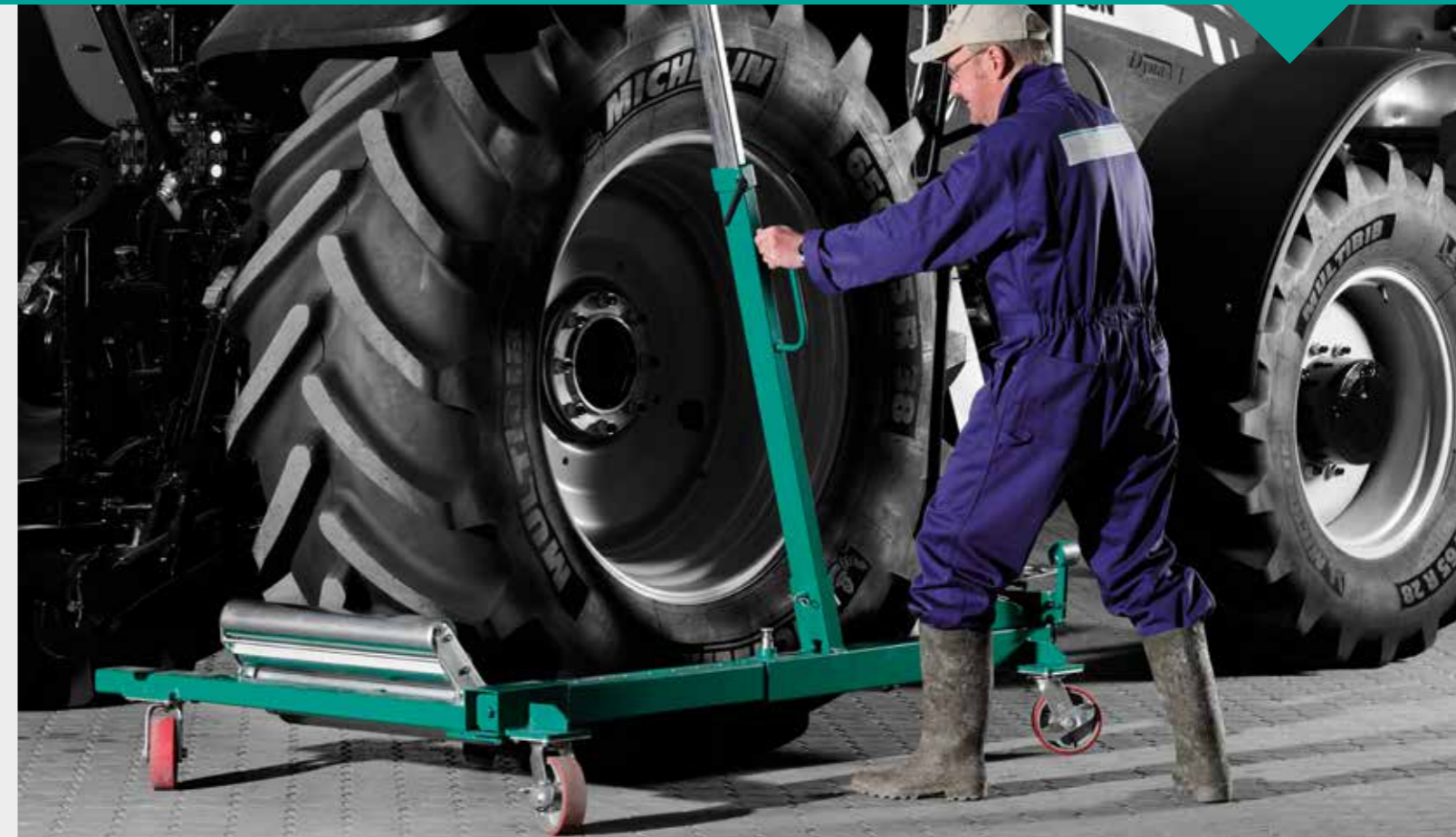
Capable of handling large wheels from 1250 mm up to 2400 mm in diameter and up to 1050 mm in width.
